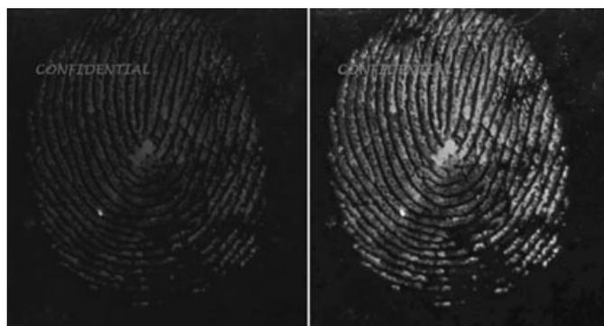
FIG. 3—Set #1. Left panel: optical photograph of a chalcogenide-glass columnar thin film grown on top of a glass slide with a sebaceous fingerprint. Right panel: the same photograph after software enhancement.
