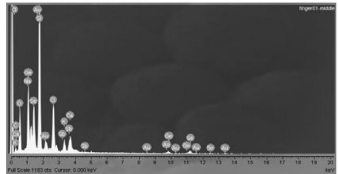
FIG. 6—Set #1. Energy-dispersive X-ray spectrum of a chalcogenide-glass columnar thin film grown on top of a glass slide with a sebaceous fingerprint.
