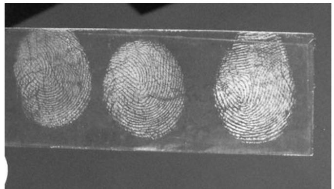
FIG. 7—Set #2. Optical photograph of a  $MgF_2$  columnar thin film deposited on three sebaceous latent fingerprints placed on a glass microscope slide.
