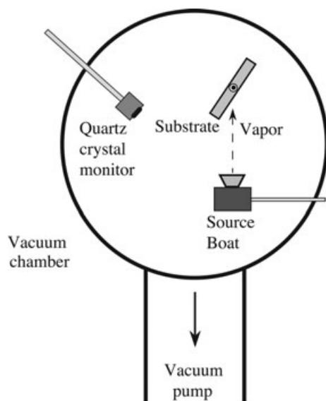
FIG. 2—Schematic of the chamber to grow columnar thin films by thermal evaporation.
