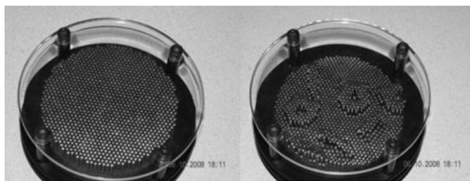
FIG. 1—Illustration of the concept using a toy called Pin Point Impression comprising parallel, identical, thin cylindrical pins. Left panel: pins over a flat surface. Right panel: pins over an undulating surface.
