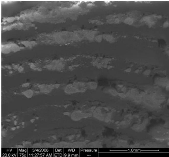
FIG. 4—Set #1. Top-surface SEM image (75 $\times$ ) of a chalcogenide-glass columnar thin film grown on top of a glass slide with a sebaceous fingerprint.
